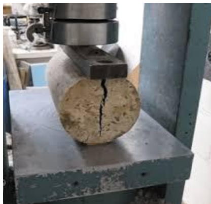
Figure-4 Split tensile test
