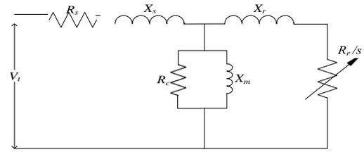
Fig. 1. Equivalent circuit of induction motor
