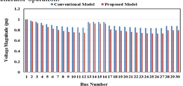
Fig. 6. Bus voltage magnitudes for the droop controlled generator operation.
