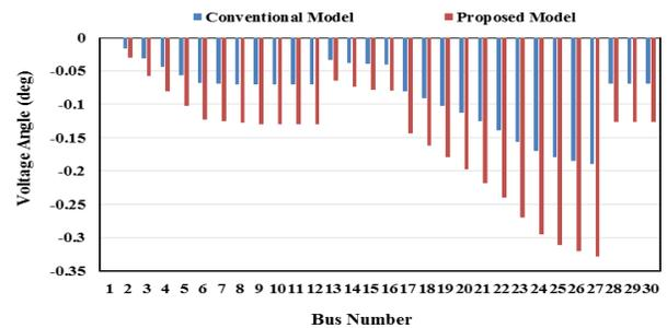
Fig. 5. Bus voltage angles for the P-V controlled generator operation.
