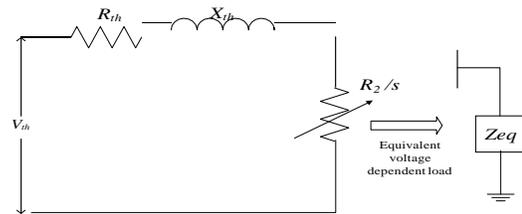
Fig. 2. Thevenin's representation of the equivalent circuit
