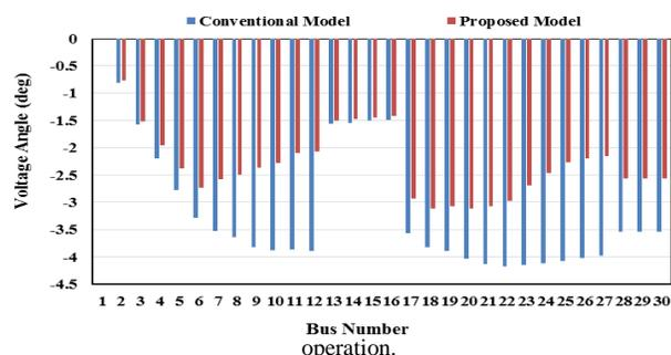
Fig. 7. Bus voltage angles for the droop controlled generator operation.
