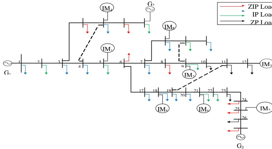
Fig. 3. 30 bus weakly meshed distribution system with induction motor and generator
