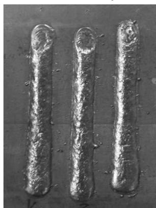
**Fig. 4.** Weld beads obtained by local cavity welding
