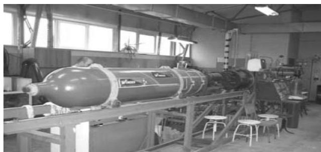
**Fig. 13. Test facility for simulating underwater welding on high depths**
