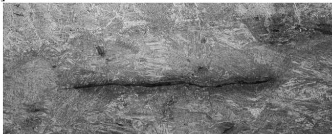
**Fig. 6.** Microphotograph of the cold crack in the bainite structure of heat affected zone [18]
