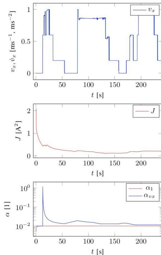
Fig. 4. Plot illustrating the model fitting on recorder d ata: Speed in x-direction; error of the model while learning; Variable Learning Rates for the model
