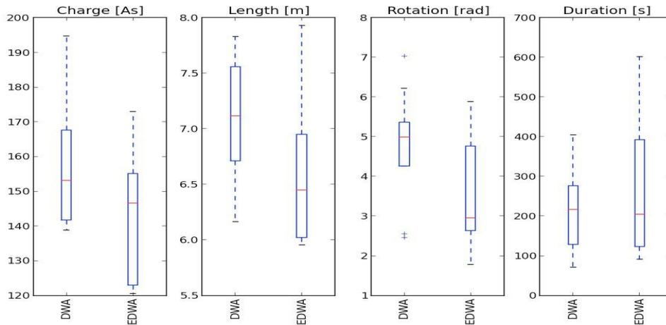
Fig. 3. Box plots indicating charge, length, rotation and duration of the test runs. Every value allows comparison between DWA and EDWA test setups.
