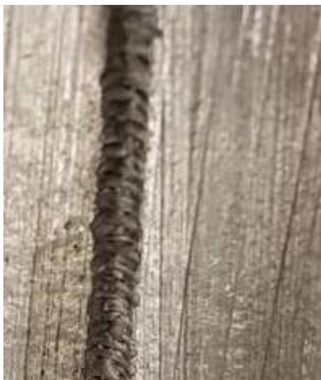
Figure 12. Welded top bead, AM 60, No Filler Material
