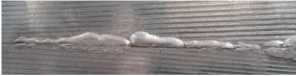
Figure 1. Mg AM 60, TIG-welded, Leaked Melt on the Reverse Side
