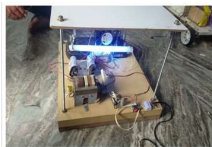
Figure 6.1 High Voltage DC generation circuit hardware prototype installation
