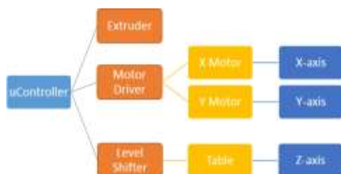
Fig.2. Flow Diagram of Control
