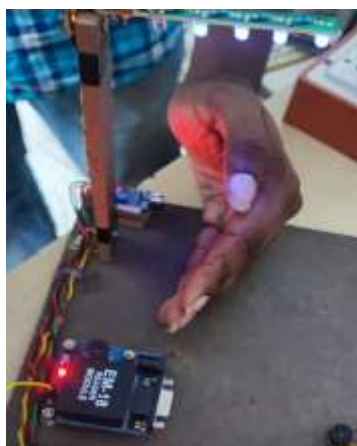
Fig13. Activation of UV light when the IR sensor detects the student's hand
