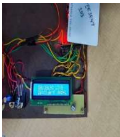
Fig12. Detection of exit when a student with ID3 places his card on the RFID reader.
