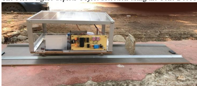
Fig 2. Tram stops as it identifies an object in its path.
