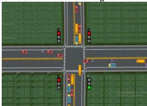
Fig. 4.3: Pygame Output Displaying Dynamic Signal Timings Based on Simulated Lane Density
