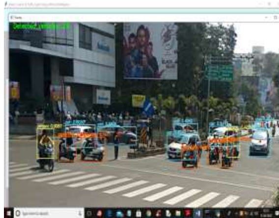
Fig. 4.8: Final Output Video Generation Post YOLO Processing with Optimized Traffic Signals
