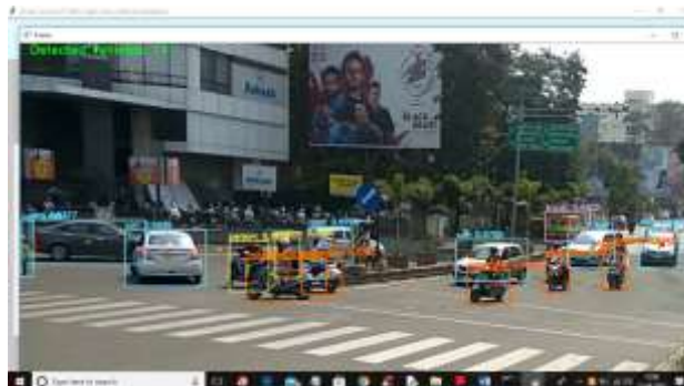
Fig. 4.6: YOLOv8 in Action: Detecting and Counting Vehicles from Uploaded Traffic Video
