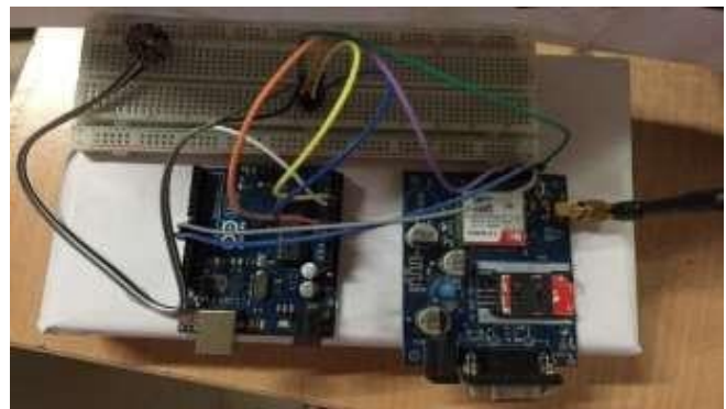
Fig. 2: Connections between sensors, Arduino and GSM modem
