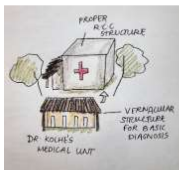
Figure 1 - Schematic diagram showing Dr. Kolhe's clinic where the basic waiting and appointment part is made out of local materials whereas, the operational and treatment part is made up of proper R.C.C.
