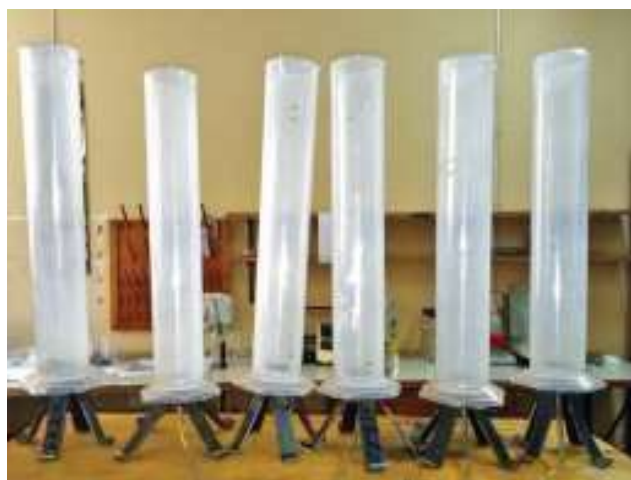
Figure 2. a) Columns used to pack biochar and sand and b) schematic drawing of column.
