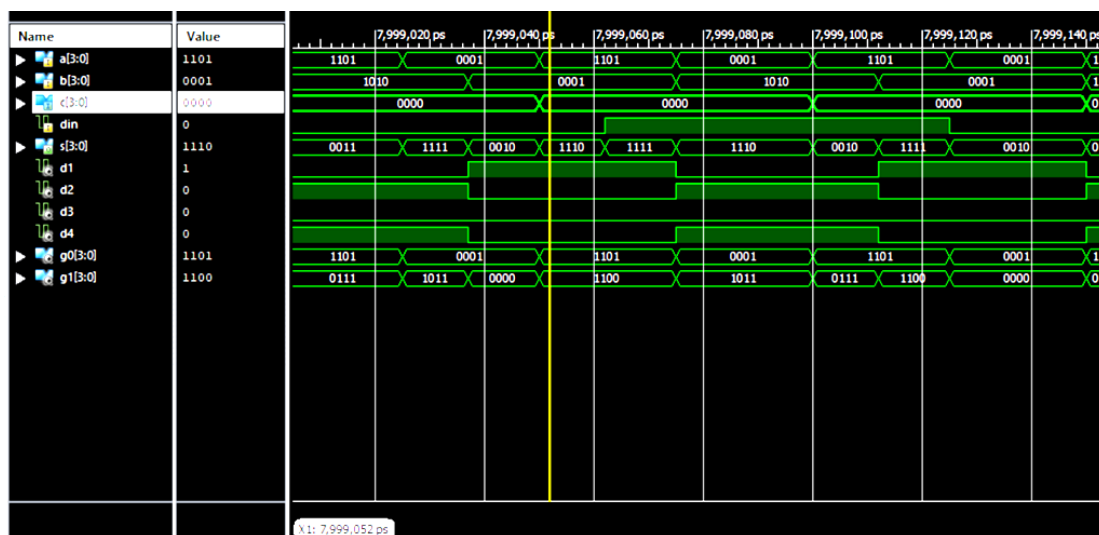
Figure 5: Simulated Output for Reversible 4-bit Parallel Adder using TSG Gate
