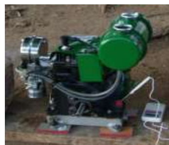
Fig 3: Single cylinder four stroke SI engine
