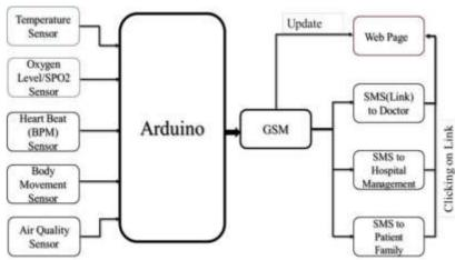
The data from Arduino to GSM will be transferred, the data in digital form. GSM-900 is used to transfer or update the data to the website and also it will send the SMS to the doctor, hospital management and family members at critical condition and abnormal condition data.
