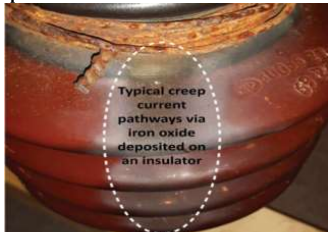
Fig :8.2 Corrosion of insulator
