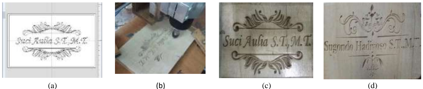
Figure 6: (a)Image design. (b)Engraving process. (c)Engraving result. (d)Engraving result.
