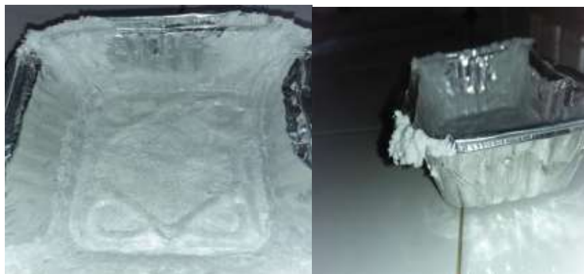
Fig: Detoriated aluminum foils upon stored with alkaline solution
