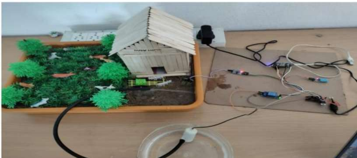
Figure -1: Experimental set up of auto irrigation system detect the rainfall in advance so that we can reduce over watering as well as water wastage.
