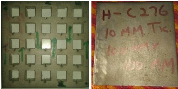
Fig.2. Workpiece After and Before Machining
