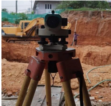
Figure 3: Auto Level Instrument
