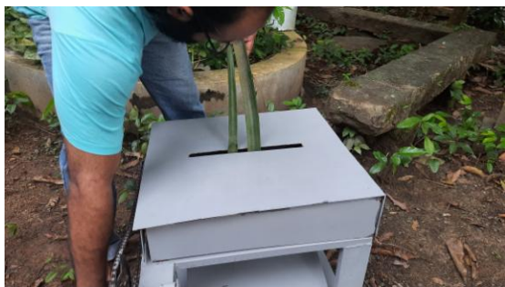
PLATE – I PROTOTYPE OF THE LOW-COST PINA DECORTICATOR – FEEDING OF PINEAPPLE LEAVES
