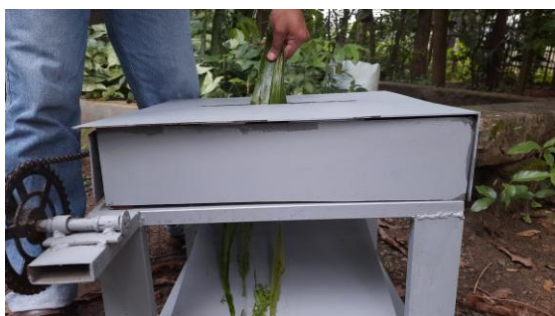
PLATE – II PROTOTYPE OF THE LOW-COST PINA DECORTICATOR – EXTRACTION OF PINA FIBRE
