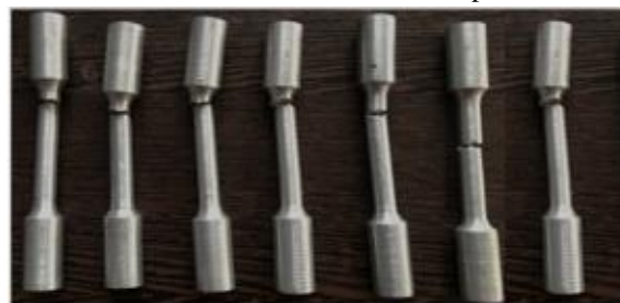
FIGURE 3. Tensile fractured specimens
