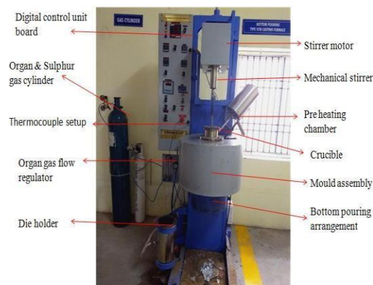
FIGURE 1. Stir Casting Setup
