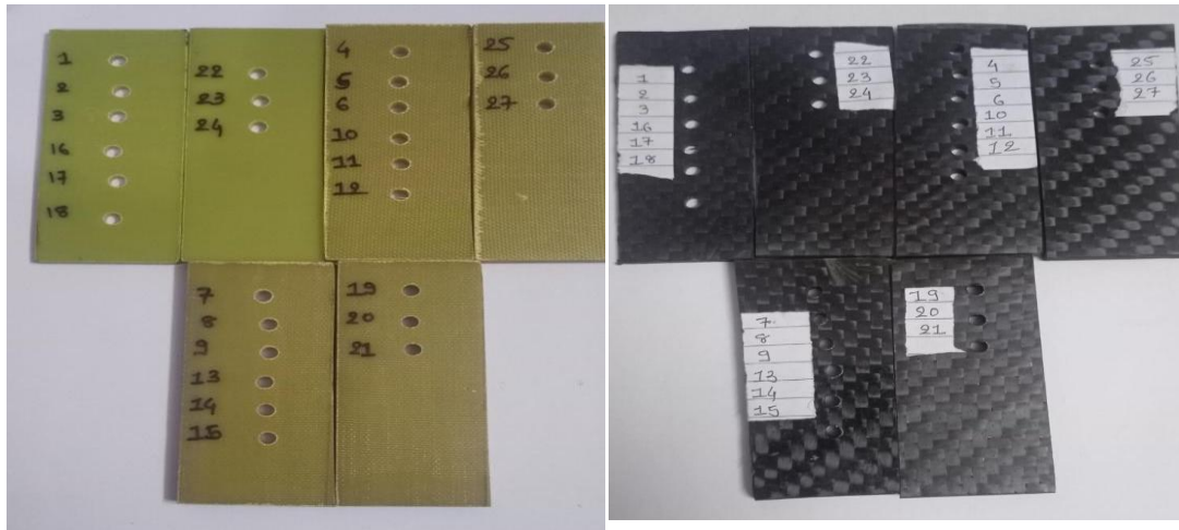
Figure 7 Photograph of GFRP & CFRP sheet drilled with 5mm bit in L27 Taguchi's Array respectively.
