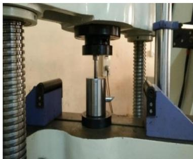
**Figure 3** ECAP Process process
