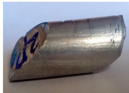
**Figure 4** Specimen after ECAP
