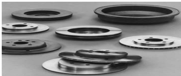
Figure 2. Discontinuously reinforced aluminum MMC brake rotors[ http://www.mmc-assess.tuwien.ac.at ]
