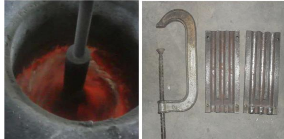
Fig. 4. Preparation of Al-5083 composite & CI permanent mould [5]
