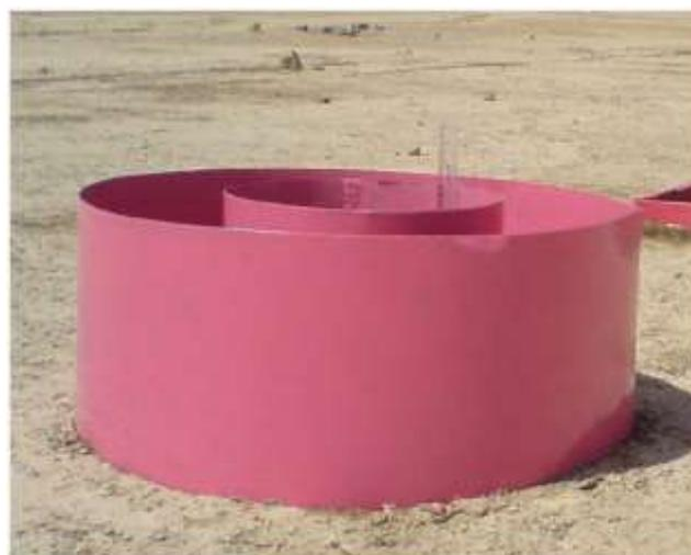
Figure 5. Double ring infiltrometer.
