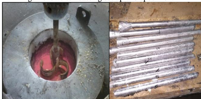
Fig. 1 Stir casting set up and specimen
