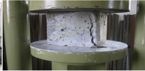
Figure 2 Specimen after fai
