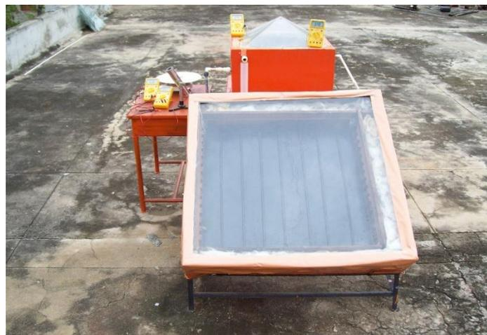
**Fig (2) Pyramid Solar Still with Flat Plate Collector**
