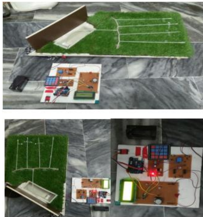
Figure 5. Hardware set up of proposed solar water pumping system.
