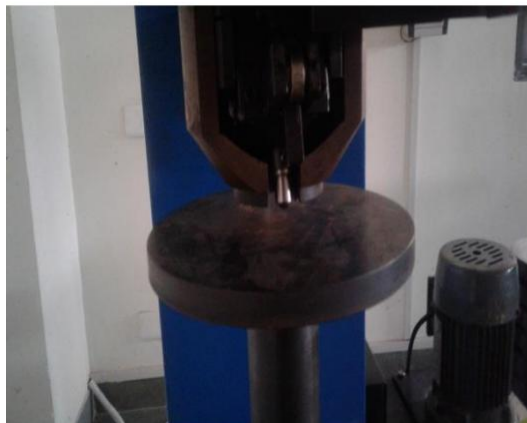
Fig 4.1: Brinell hardness testing
