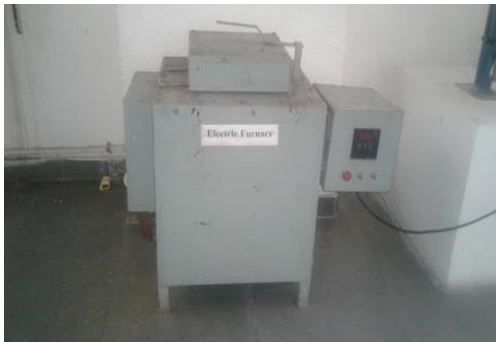
Fig 2.2 Electric furnace for melting alumina
