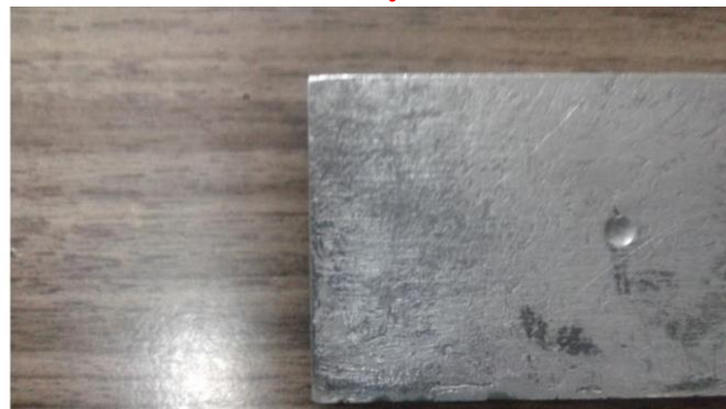
Fig 4.3: A sample showing indentation
