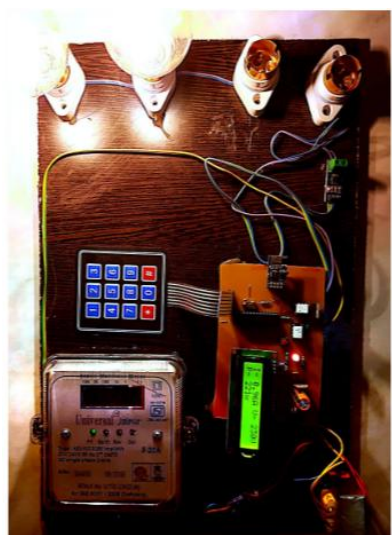
Figure 3.3: Two bulbs of 100W connected resulting in 200W
