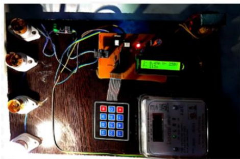
Figure 3.2: Threshold power set to 300W, 100W bulb is connected
